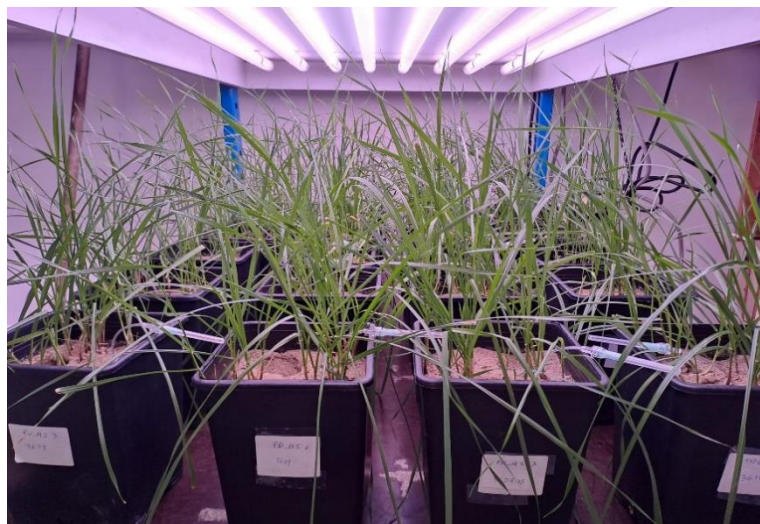
Figure 2 – Pots of ryegrass with BBFs in river sand as soil, maintained for 13 weeks, for the evaluation of the BBFs as potential alternative P-rich fertilizers to the commercial mineral fertilizer TSP.
