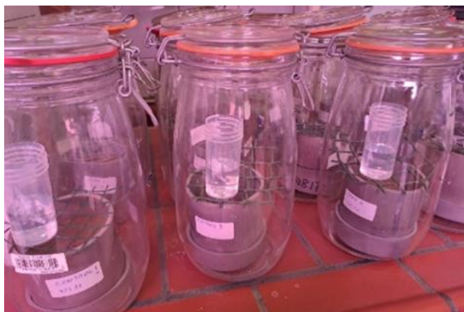
Figure 3 - Carbon mineralization setup for 92 days: PVC tubes filled with soil and organic carbon-rich products, with the addition of a NaOH vial to trap the CO 2 emitted by the microorganisms, for the assessment of these products as potential soil enhancers. These jars were maintained in the dark throughout the experiment.
